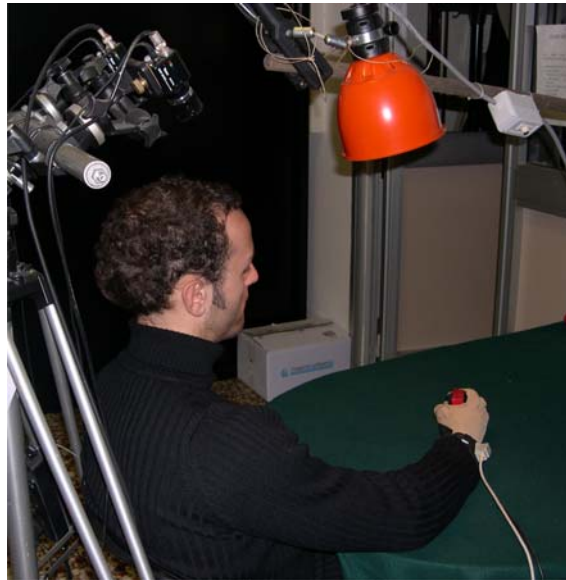
Figure 7: The recording setup. The user wears the cyber glove and reaches for an object. Cameras in this image are placed behind the person and see a good portion of the table. The visual environment
